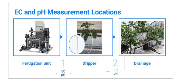
If the measurement shows an accumulation of salts beyond a predetermined limit (usually 0.5mS), a rapid response is necessary to prevent damage
