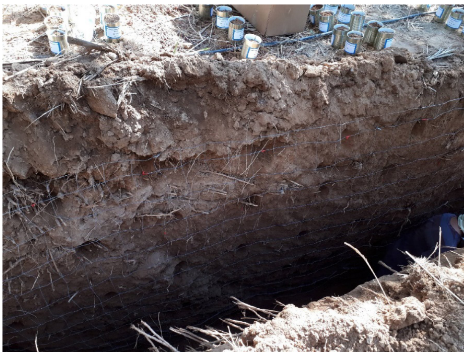
Image 4: The sampling pit with the coordinate grid and the central root layer 30-60 cm deep.
